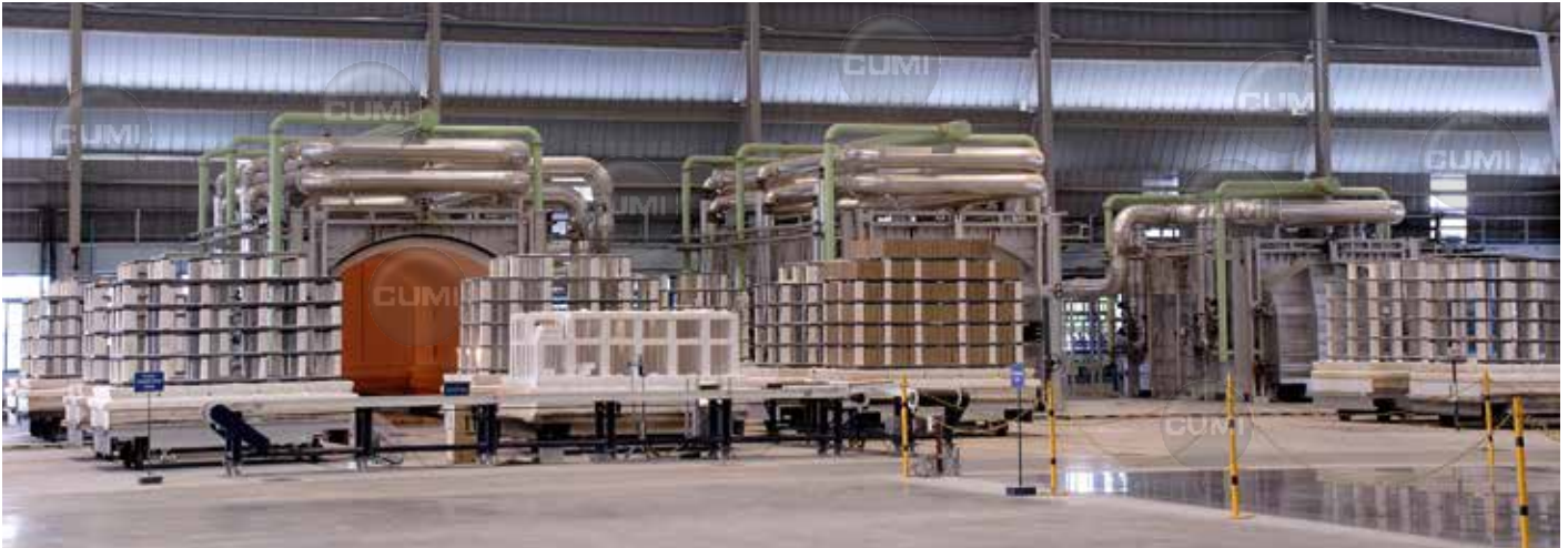
Batch Kilns with operating Temp. upto 1750°C
